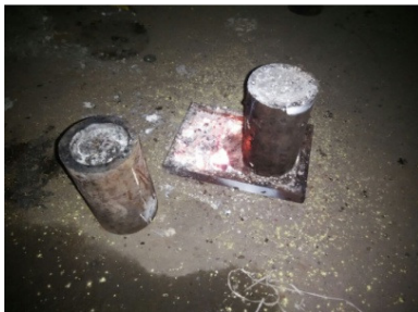
Figure 4: Casting MMC is poured in Die
