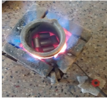
Figure 2: Mg rods being heated in furnace
