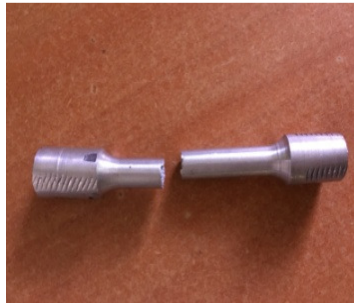
Figure 7: Tensile Specimen after testing
