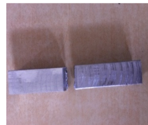
Figure 9: Impact Specimen after Testing
