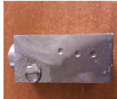
Figure 8: Hardness Specimen after Testing
