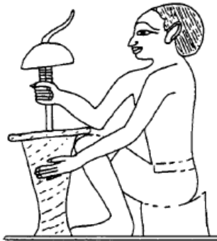
Fig.13 Modified boring drill at the 18 th dynasty [19].
