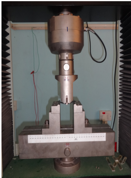
Figure 2. Flexural Test Setup
