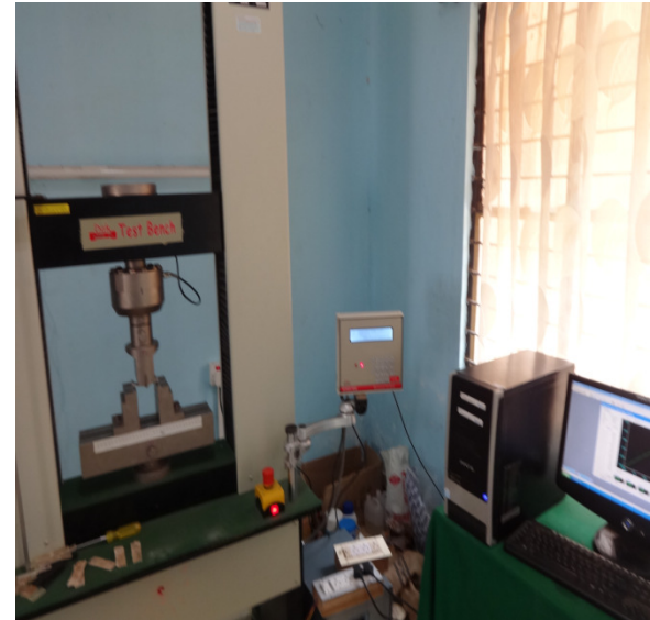
Figure 2. Flexural Test Setup
