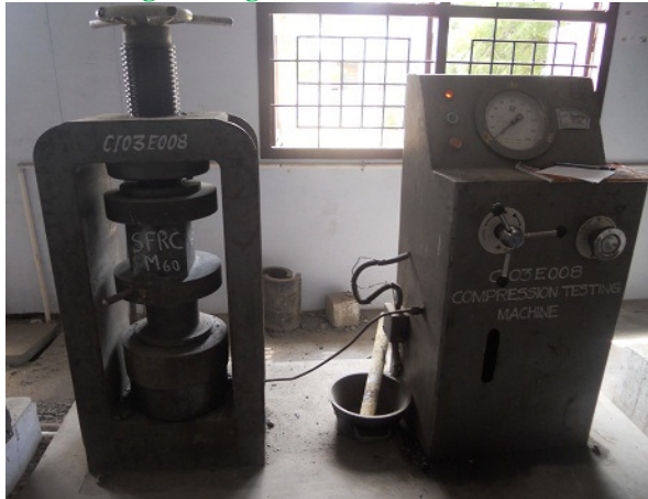
Compressive Strength Testing
