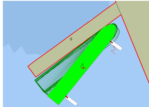
Fig.6. Ship's Pull By Tugs, Using Push/Pull Method
