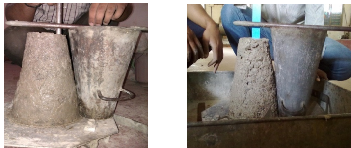
Fig 3.1:- Slump of Fresh Geopolymer and OPC Concrete
