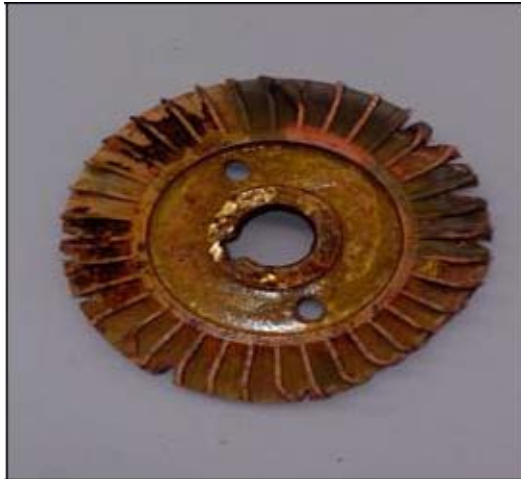
Fig. 2: The Damaged Impeller
