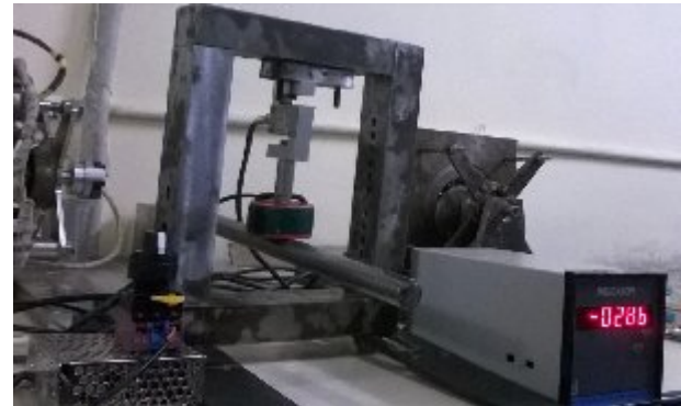
Fig. 6) Gap between the electromagnet and shaft is ZERO with an impulse on shaft at static condition.
