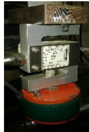
Fig. 1) Assembly showing electromagnet and S-type load cell.
