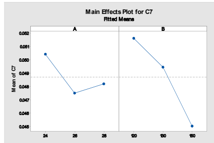
Figure 10 Main effect of end face finish
